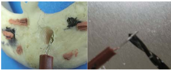
Fig 1 Temperature measurement method by thermocouple element with an insulating tube.
